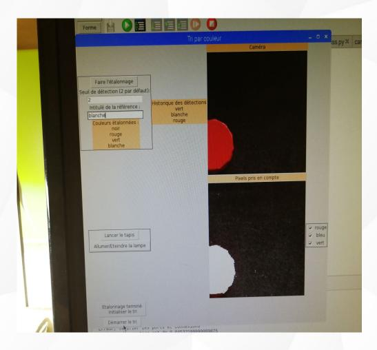
In the software section, they used Python to write programs that can recognize objects based on color and shape, can control the light source and the transmission device through the nucleo 1,We learned Python, including various libraries and code structures.
