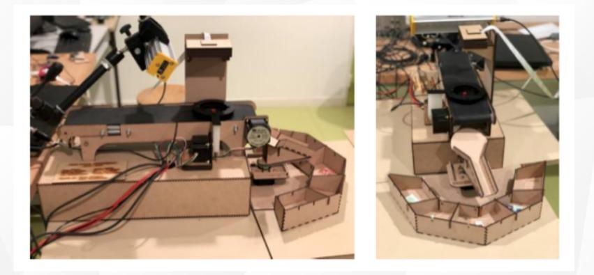
The hardware part is mainly composed of five parts, Raspberry camera, lighting, transmission track, sorter, receiving box.
