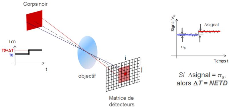
**Figure 4.2:** Illustration of the concept of NETD.
