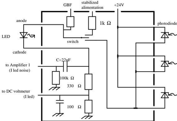
**Figure 1.10:** Setup of the sub-Poissonian/Poissonian light emitting device
