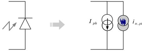
**Figure 1.6:** Photodetection noise model.
