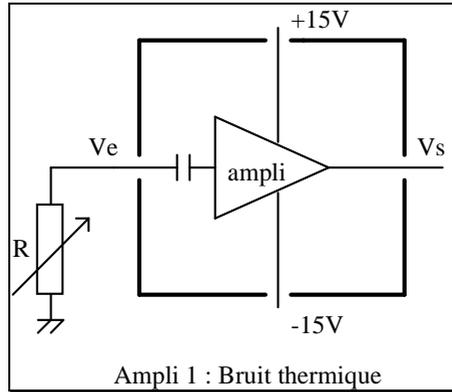
**Figure 1.3:** Amplifier noise and thermal noise measurements circuit.
