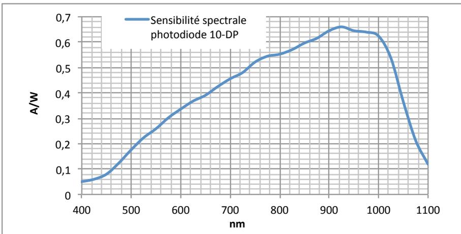
**Figure 3.6:** Spectral response of the calibration photodiode
