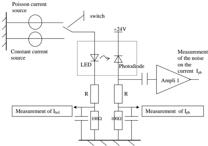
**Figure 1.9:** Principle of the shot-noise reduction experiment
