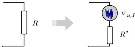
**Figure 1.4:** Resistance thermal noise model
