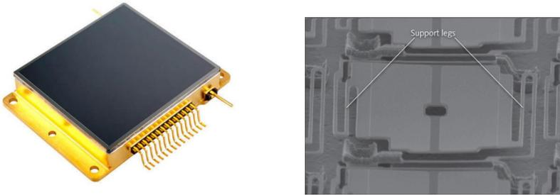
**Figure 4.1:** Left : Microbolometer Focal Plane Array (credit : [www.ulis-ir.com](http://www.ulis-ir.com)). Right: a pixel (credit : <http://www.laserfocusworld.com>).
