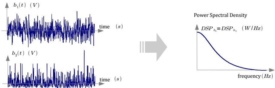
**Figure 1.1:** Two different noises with the same PSD.
