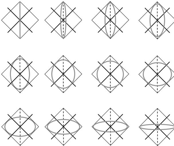
**Figure 4.7** – Resulting ellipses with respect to the dephasing introduced by the birefringent plate. The incident polarisation is represented by a bold grey line when the phase is null and dashed otherwise. Its orientation stands at  $45^\circ$  from the neutral axes of the plate appearing in bold black lines.
