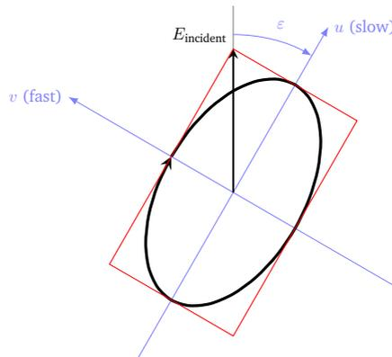
**Figure 4.5** – Ellipse at the output of a quarter wave plate for a linear input polarisation. The ellipticity is indeed the angle between the direction of the input polarisation and the neutral axis of the QWP.
