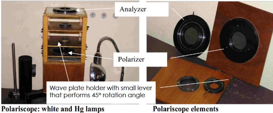
**Figure 1.1** – The different components of a polariscope.
