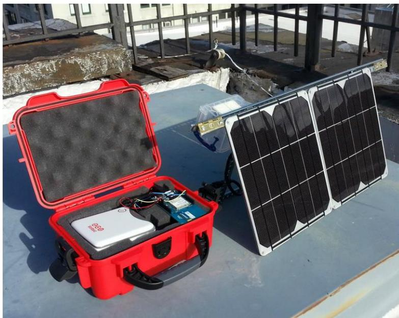
*Powering the sensor with solar panels to go to the field.*
