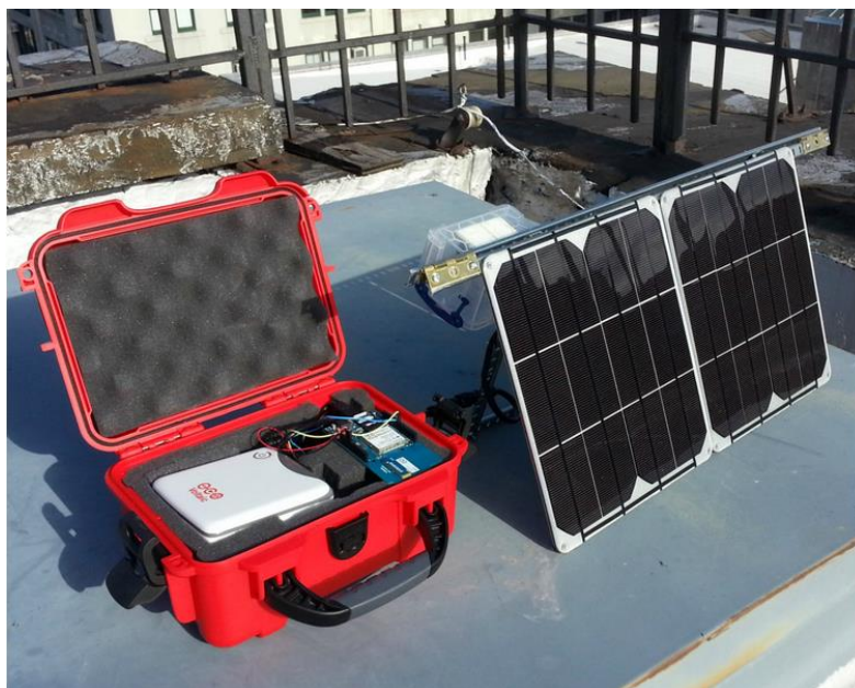
Powering the sensor with solar panels to go to the field.
